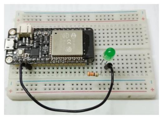
Here we connect an LED circuit in the **GPIO21** by connecting a 330ohm resistor to GPIO21. The other end of the resistor goes to the positive of the LED and then black wire to ground the LED.
