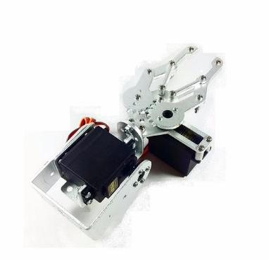
The Robotic Arm 2 Degrees of Freedom is a robotic arm kit that offers a manipulator claw and bracket made in aluminum. It has two degrees of freedom, one is for controlling the arm, the other the rotation of the arm. The kit is also easy to construct, and could be done by yourself.
