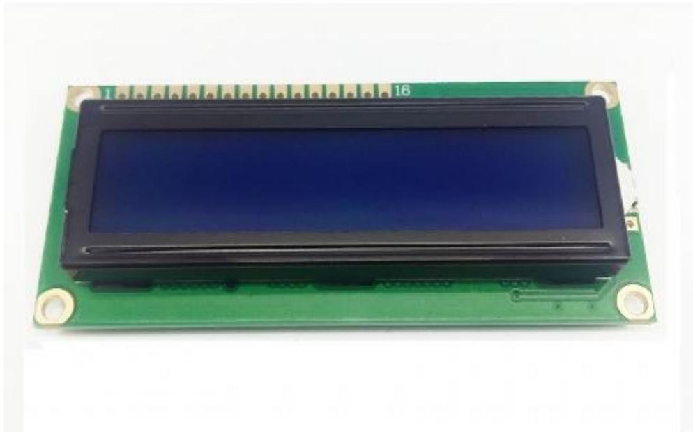
The LCD Module is a display module for displaying data, be it in the form of numbers, texts or symbols. You can display 16 characters in a single row, with two rows available.
