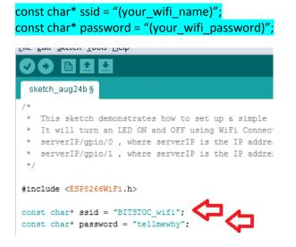
After setting up your WiFi name and password in the code, **Compile and Upload the code** to the board. Now open the Serial Monitor from the Arduino IDE by clicking the magnifying glass button at the upper right corner. When you open the Serial Monitor set the **baud to 115200**. Copy the IP Address shown in your Serial monitor in this case its **192.168.43.230**. You should see an output like the one below.
