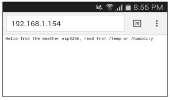
In order to get the temperature and humidity to be displayed, type in the keyword **/temp** or **/humidity** after the IP\_Address.
