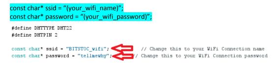
After setting up your WiFi name and password in the code, **Compile and Upload the code** to the board. Now open the **Serial Monitor** from the Arduino IDE by clicking the magnifying glass button at the upper right corner. When you open the Serial Monitor set the **baud to 115200.** Copy the IP Address shown in your Serial monitor in this case its **192.168.1.154**. You should see an output like the one below.
